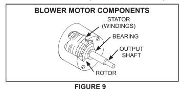
The controller uses sensing devices to sense what position the rotor is in at any given time. By sensing the position of the rotor and then switching the motor windings on and off in sequence, the rotor shaft turns the blower.
