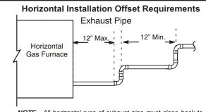
**NOTE -** All horizontal runs of exhaust pipe must slope back toward unit. A minimum of 1/4" (6mm) drop for each 12" (305mm) of horizontal run is mandatory for drainage.
