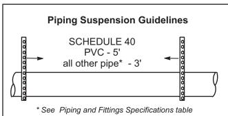
**NOTE** - Isolate piping at the point where it exits the outside wall or roof in order to prevent transmission of vibration to the structure.
