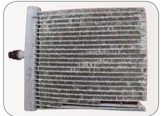
*Figure 8: E-Coated Sample After Testing*
