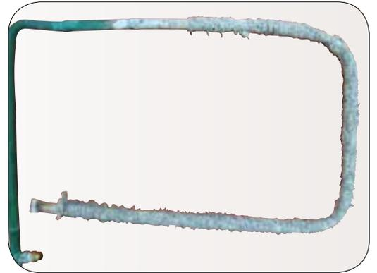
*Figure 7: Uncoated Sample After Testing*
