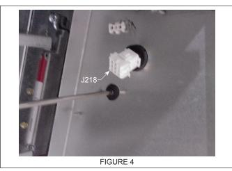
5. Install provided adapter panel using existing screws that were removed in **Step 2**.
