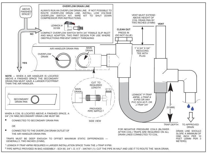
FIGURE 6. Typical Main and Overflow Drain
