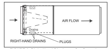
FIGURE 2. Right-Hand Discharge Configuration
