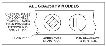
**FIGURE 8. Drain Line Connections**
