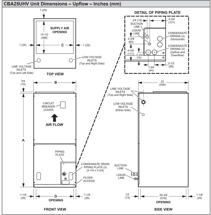
**NOTE** – Unit is shipped configured for horizontal right-hand air discharge. Unit may be converted to horizontal left-hand air discharge by repositioning horizontal drain pan. Dimensions remain the same in all configurations.
