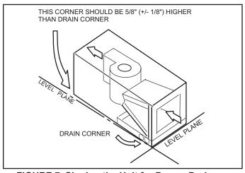
FIGURE 7. Sloping the Unit for Proper Drainage
