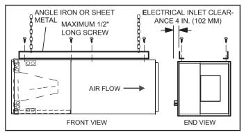
FIGURE 3. Suspending Horizontal Unit LEFT-HAND AIR DISCHARGE
