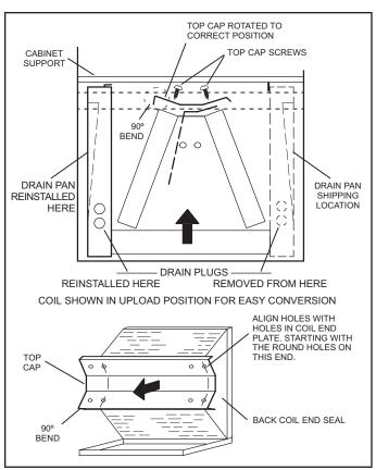
FIGURE 4. Field Modification for Left-Hand Discharge
