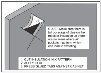
FIGURE 17. Repairing Insulation
