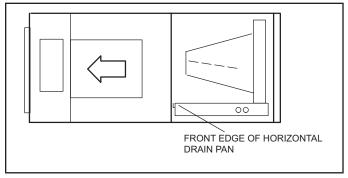
FIGURE 5. Left-Hand Discharge Configuration
