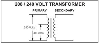
FIGURE 13. Converting Unit from 240VAC to 208VAC
