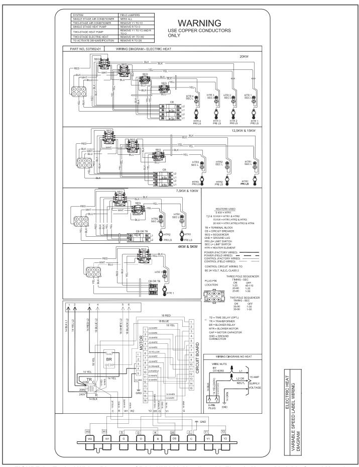
FIGURE 14. Typical Wiring Diagram – CBA25UHV Air Handler with Electric Heat – (Variable-Speed Motor)
