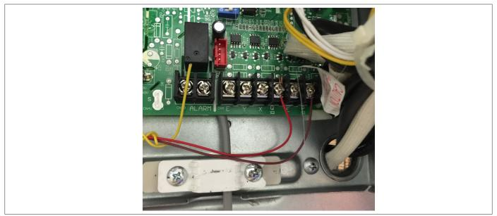
Figure 16. Alarm Device Connection Points (Typical)
