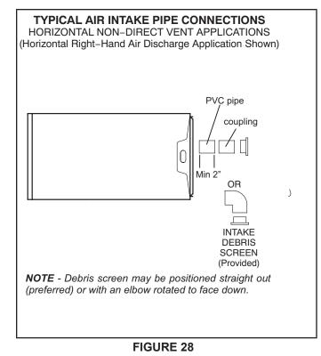
Follow the next two steps when installing the unit in Non-Direct Vent applications where combustion air is taken from indoors or ventilated attic or crawlspace and flue gases are discharged outdoors.
