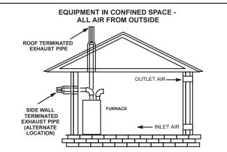
**NOTE-**Each air duct opening shall have a free area of at least one square inch per 2,000 Btu (645mm<sup>2</sup>per .59kW) per hour of the total input rating of all equipment in the enclosure. If the equipment room is located against an outside wall and the air openings communicate directly with the outdoors, each opening shall have a free area of at least 1 square inch per 4,000 Btu (645mm<sup>2</sup> per 1.17kW) per hour of the total input rating of all other equipment in the enclosure.
