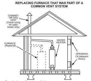
If replacing a furnace which was
