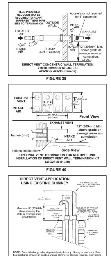
inside chimney until the pipe open end is above top of chimney and terminate as illustrated. In any exterior portion of chimney, the exhaust vent must be insulated.
