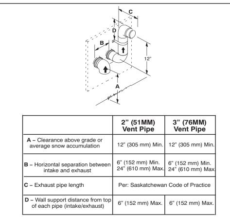
**NOTE** – Flue gas may be acidic and may adversely affect some building materials. If flue gases impinge on the building materials, a corrosion-resistant shield should be used to protect the wall surface. The shield should be constructed using wood, sheet metal or other suitable material. All seams, joints, cracks, etc. in affected area, should be sealed using an appropriate sealant.
