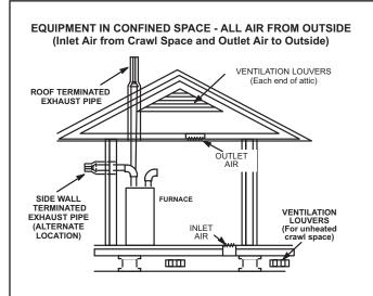
**NOTE**-The inlet and outlet air openings shall each have a free area of at least one square inch per 4,000 Btu (645mm<sup>2</sup> per 1.17kW) per hour of the total input rating of all equipment in the enclosure.
