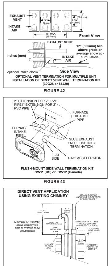
NOTE - Do not discharge exhaust gases directly into any chimney or vent stack. If vertical discharge through an existing unused chimney or stack is required, insert piping inside chimney until the pipe open end is above top of chimney and terminate as illustrated. In any exterior portion of chimney, the exhaust vent must be insulated.
