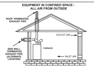
**NOTE**-Each air duct opening shall have a free area of at least one square inch per 2,000 Btu (645mm<sup>2</sup>per .59kW) per hour of the total input rating of all equipment in the enclosure. If the equipment room is located against an outside wall and the air openings communicate directly with the outdoors, each opening shall have a free area of at least 1 square inch per 4,000 Btu (645mm<sup>2</sup> per 1.17kW) per hour of the total input rating of all other equipment in the enclosure.
