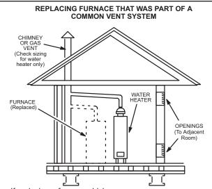
If replacing a furnace which was commonly vented with another gas appliance, the size of the existing vent pipe for that gas appliance must be checked. Without the heat of the original furnace flue products, the existing vent pipe is probably oversized for the single water heater or other appliance. The vent should be checked for proper draw with the remaining appliance.
