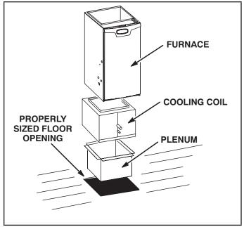
FIGURE 16 Return Air Opening -- Downflow Units
